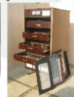
DRYER WITH DRAWERS AND TRAYS Drying of flower seed and small amounts of basic seed
